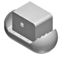
TCG provides accurate line temperature and conductor information, and uses the magnetic field on the transmission line to generate the required power. Also, there are some energy storage devices inside the TCG, so even if the power of a transmission line is insufficient or the power supply in interrupted, TCG can still operate stably.
